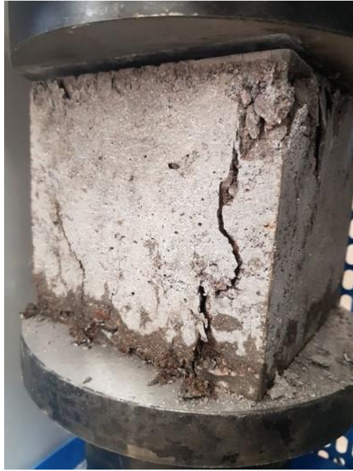
Figure 3. Failure of a concrete specimen
