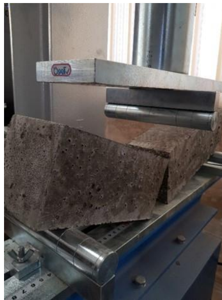
Figure 7 Broken concrete beam during a flexural strength test
