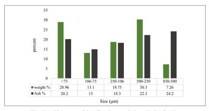
Fig. 2. Ash¹ content of the gilsonite sample in each size fraction
