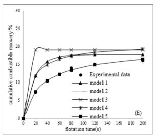
Fig. 5. Fitting the first order kinetic model on the data derived from different size fractions in rougher flotation (A) -850+500, (B) -500+250, (C) -250+106, (D) -106+75, (E)  $<75 \mu m$
