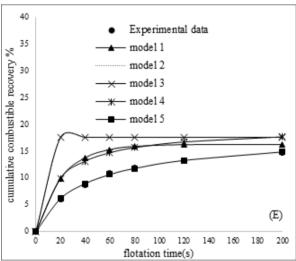
Fig. 6. Fitting the first order kinetic model on the data derived from different size fractions in cleaner flotation (A) -850+500, (B) -500+250, (C) -250+106, (D) -106+75, (E)  $<75 \mu m$
