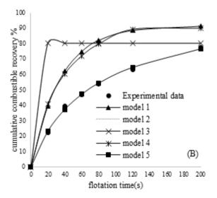
Fig. 4. Fitness of the kinetic models to (a) petroleum-MIBC and (b) absence of collector and frother flotation tests
