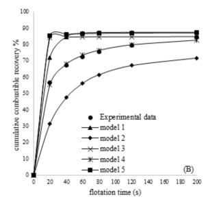
Fig. 3. Fitness of the kinetic models to (A) petroleum-MIBC and (B) absence of collector and frother flotation tests
