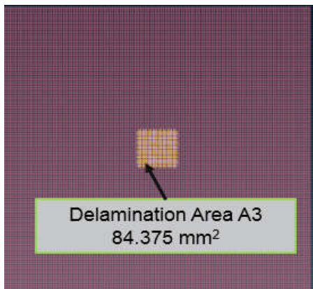
Fig. 3. Top view of delamination incorporated.
