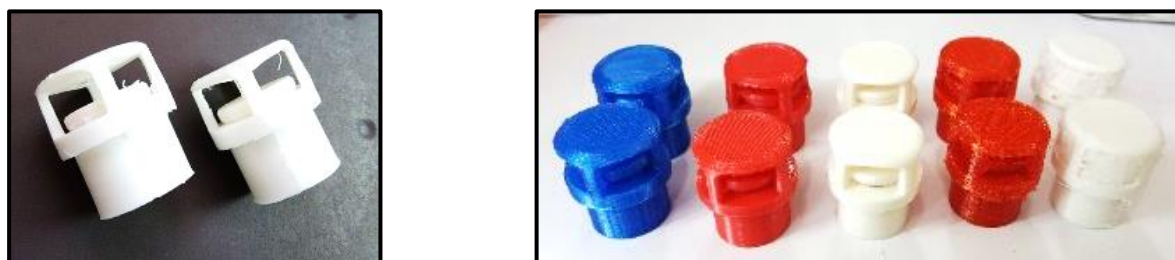
Fig. 7. The 3D printing of artificial single leaflet mechanical heart valve
