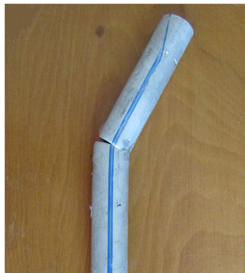
Fig. 10. Fractured AA 6063-T6 tube after (a) simulation and (b) experimental bending test at a bending radius of 32.5 mm.
