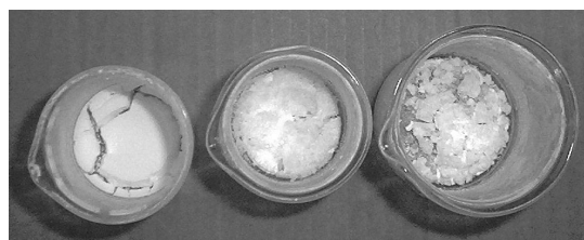
Fig. 4. The xerogel morphology in different acid concentrations. Higher amount (right side) neutral condition (center), and lower amount of acid (left side).
