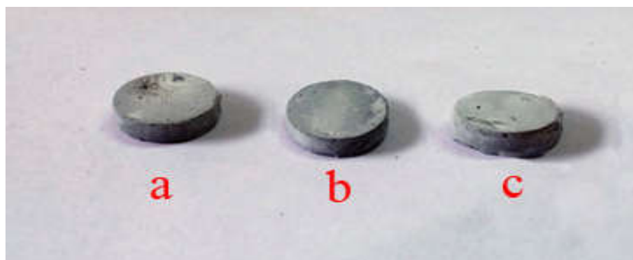
Fig. 4. Illustration of samples after nitriding in different temperature a) 1275 C b) 1300 C c) 1325 C
