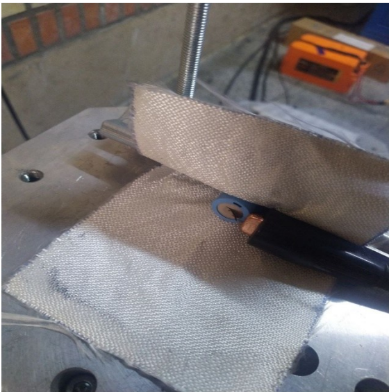
Figure 1: Orientation of the cylindrical 18650 lithium-ion battery and applied random vibration axes (X, Y, and Z) in accordance with the IEC 62660-2 standard.
