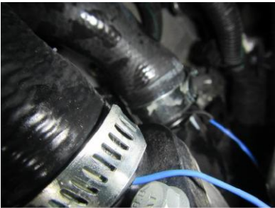
Figure 4: The inlet and outlet air temperature sensors of fan on the vehicle
