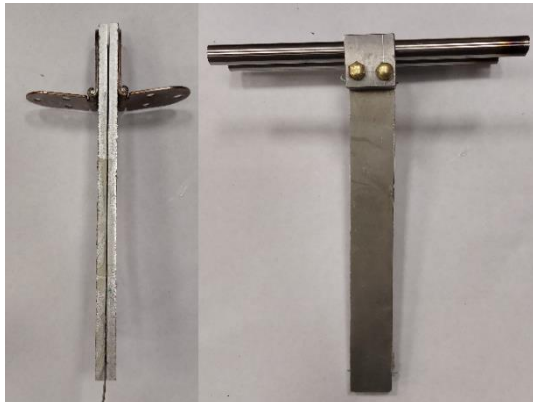
Figure 5: Specimens for static and impact loading
