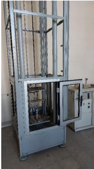
Figure 8: DCB impact test setup.
