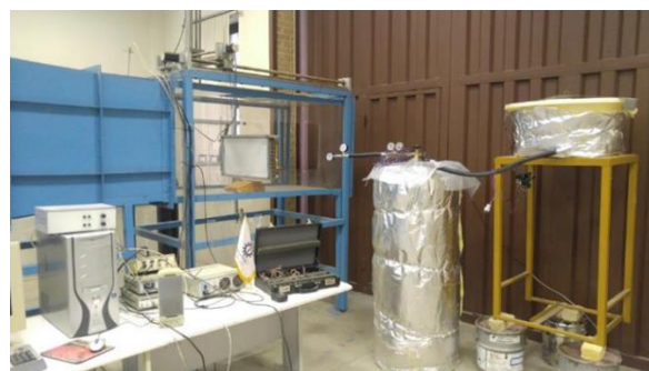
Figure 3: The wind tunnel and the condenser testing apparatus.
