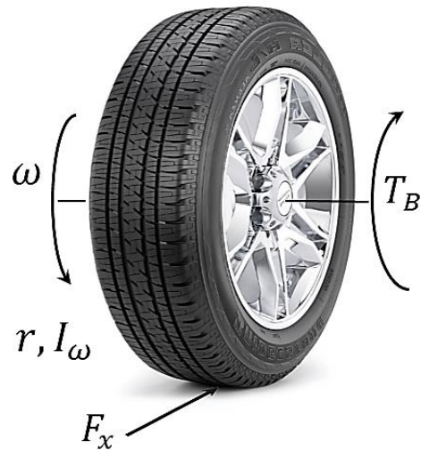
Figure 3: Free body diagram of the wheel during braking
