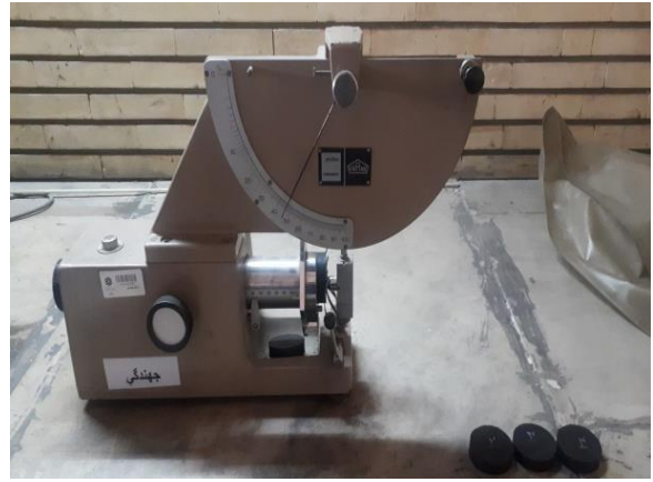
Figure 15: Rubber resilience device
