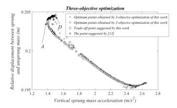
Fig10. Pareto front of vertical sprung mass acceleration and relative displacement between sprung and unsprung mass resulted by 3objective optimization for case 1.
