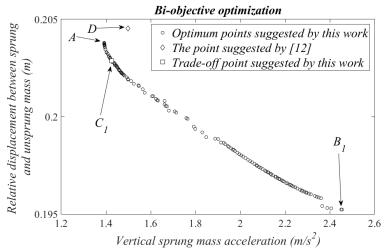
Fig6.Pareto front of vertical sprung mass acceleration and relative displacement between sprung and unspring mass resulted by bi-objective optimization for case 1.
