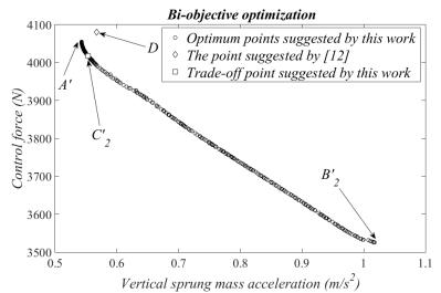
Fig8. Pareto front of vertical sprung mass acceleration and relative displacement between sprung and unspring mass resulted by bi-objective optimization for case 2.
