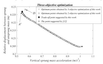
Fig12. Pareto front of vertical sprung mass acceleration and relative displacement between sprung and unsprung mass resulted by 3-objective optimization for case 2.
