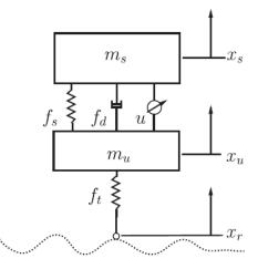
Fig2. Non-linear vehicle model [12].
