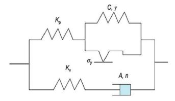
Fig4. The two-layer viscoelasticity model [32].
