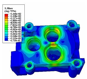
Fig11. The Von-Mises stress distribution at the end of the second stage of mechanical loading[39].
