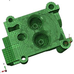
Fig5. The meshed cylinder head [38].
