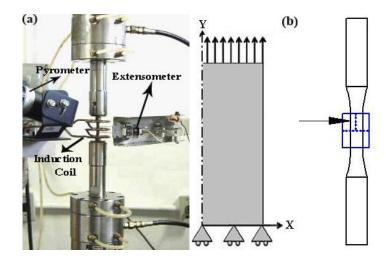
Fig3. (a) tensile test equipment and (b) The schematic view of the model for the FE simulation.
