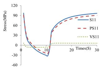
Fig12. The normal, plastic and viscous stresses in the X direction for point 1 of element 50152 versus time.
