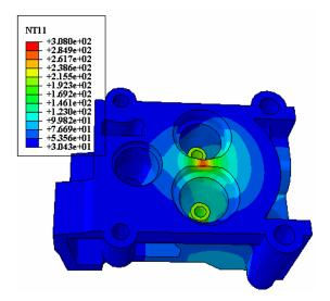
Fig8. The temperature distribution in the cylinder head.
