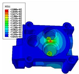
**Fig10.** The temperature distribution in the cylinder head[39].
