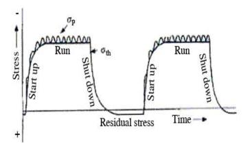
Fig1. The cyclic loading of cylinder head [20].
