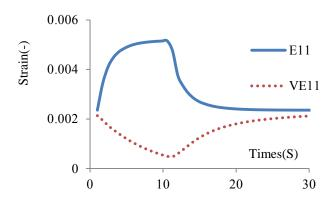
Fig15. The elastic and viscous strain for point 1 of element 50152 versus time
