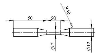
$\label{Fig2.} \textbf{Fig2.} \ \ \textbf{The tensile specimen geometry and its dimensions (in mm)}.$
