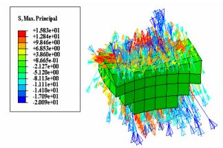
Fig13. The maximum principal stress vectors in the valve bridge when engine running (in tenth second).
