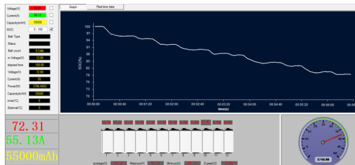
Fig.36. Battery state of charge resulted from practical test by not installing the rear spoiler
