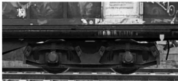
Fig2. Parabolic suspension system employed in a freight wagon
