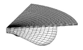
Fig3. Computational grid showing piston bowl geometry of the Caterpillar SCOTE engine
