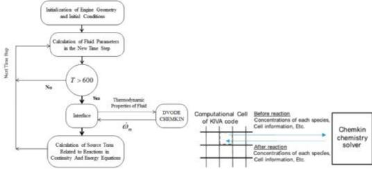
Fig4. Flowchart and diagram of coupled KIVA-CHEMKIN-DVODE model
