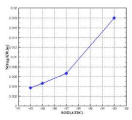
Fig16. Variation of NOx emissions over SOI-2 timing sweep
