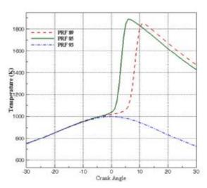
Fig8. Predicted in-cylinder temperature history for various PRF numbers
