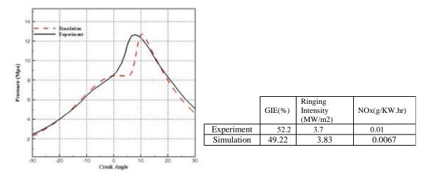
Fig5. Comparison of measured and predicted in-cylinder pressure history, GIE, RI and NOx emissions for RCCI operation
