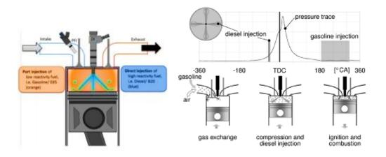
Fig2. RCCI combustion strategy and concept with different fuel characteristics [13,14]
