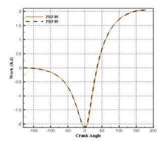
Fig7. Indicated work versus crank angle at two different PRF number
