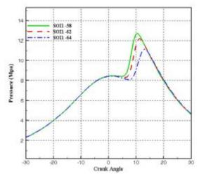
Fig10. Predicted in-cylinder pressure history over SOI-1 timing sweep
