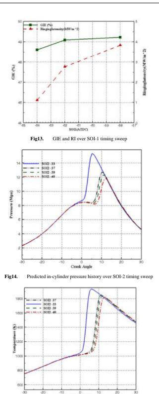
Crank Angle Fig15. Predicted in-cylinder temperature history over SOI-2 timing sweep
