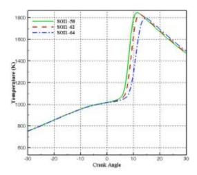
Fig12. Predicted in-cylinder temperature history over SOI-1 timing sweep
