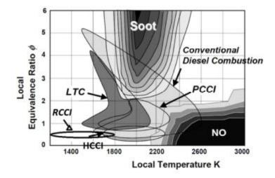
Fig1.RCCI, PCCI, LTC, HCCI and CDC operating regimes plotted on  $f^{-T}$  diagram space adapted from the work of Neely et al. and Kokjohn et al. [8,9]
