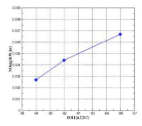
Fig11. Variation of NOx emissions over SOI-1 timing sweep
