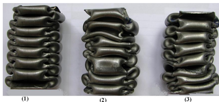
Fig5. Tested steel tubes after bearing
