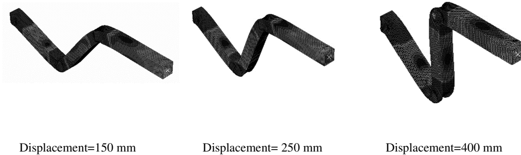
Fig12. shape of deformation of the S-rail with geometries of R=550 mm , q=25 , W=50 mm and t=2 mm at end displacement of 150, 250 and 400 mm.
