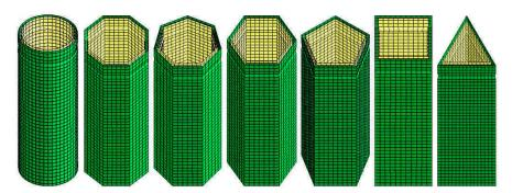
Fig2. Geometric models of hybrid tubes
