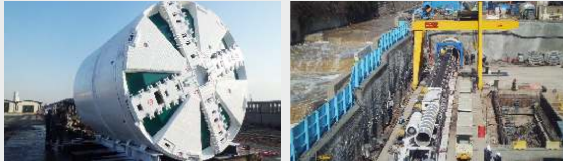
Lovat Made, EPB TBM, ME 170SE, Φ 4300 mm, Tunnel Length≈ 4000 meter
