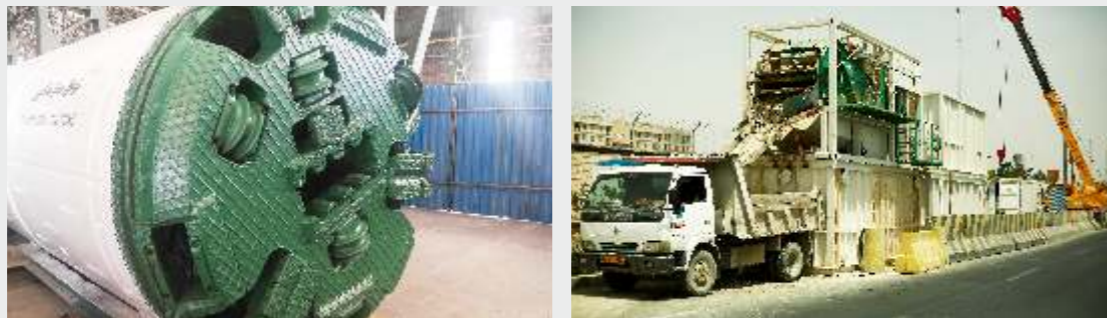
HK Made, MTBM, AVN 1600 mm, Tunnel Length≈ 2500 meter
